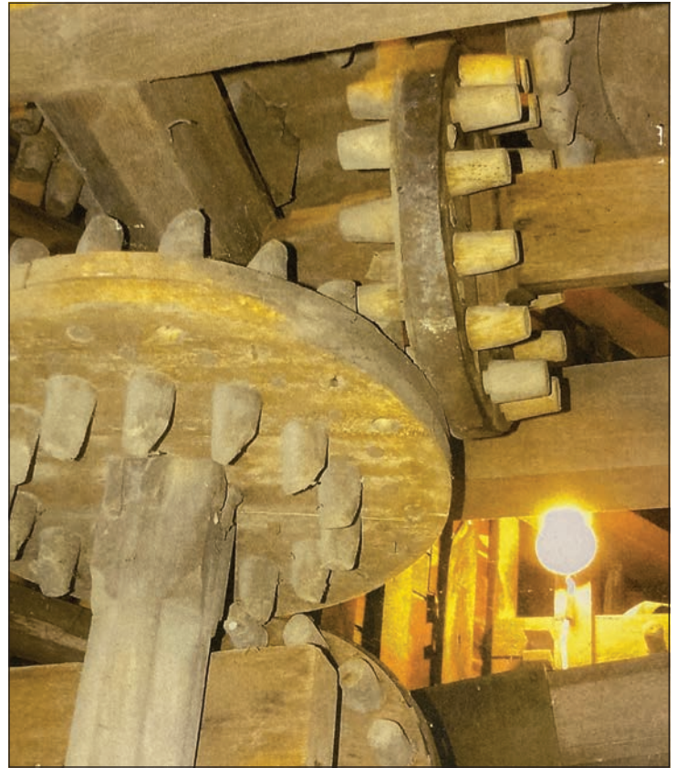
A SHAFT PROVIDED POWER to second and third floor elevators and finishing flour equipment in this 1818 mill.
