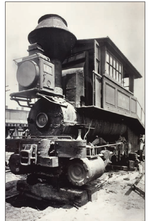
END OF THE LINE — Camel 143, built in 1863, with wheels and side rods missing, is being cut up for scrap in 1893. It's boiler blew up in 1872, killing the engineer and firemen.
