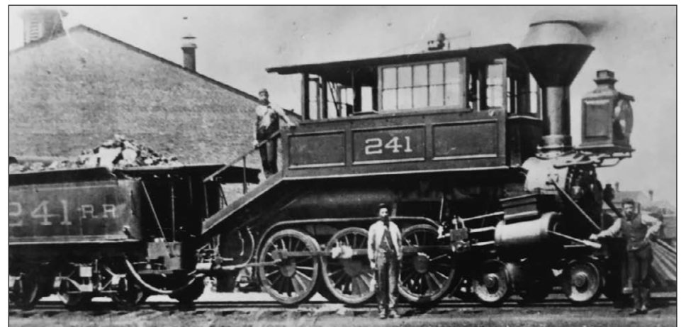
A TEN-WHEEL DAVIS CAMEL BACK #241 was built by the B&O in 1872. The picture was taken in 1886 at Willard Yards.
