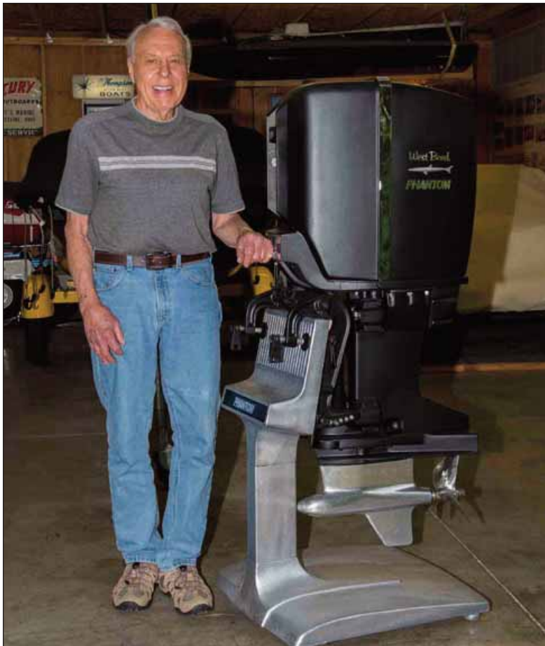
JOHN SCHEURER , a Class of 1958 Madison graduate, built a one-of-a-kind outboard motor. Starting with a photo of a model, Scheurer said, "I was inspired to put together this concept West Bend by reading a clip by former outboard motor builder Karl Reliant. From that photo I made a full-size running Phantom. The Phantom used the stock 4 cylinder 80 hp West Bend Tiger Shark engine which matched a Mercury outboard big horsepower motor of the early 1960 era."
