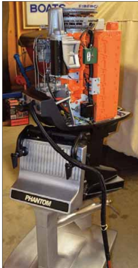
JOHN SCHEURER , a Class of 1958 Madison graduate, built a one-of-a-kind outboard motor. Starting with a photo of a model, Scheurer said, "I was inspired to put together this concept West Bend by reading a clip by former outboard motor builder Karl Reliant. From that photo I made a full-size running Phantom. The Phantom used the stock 4 cylinder 80 hp West Bend Tiger Shark engine which matched a Mercury outboard big horsepower motor of the early 1960 era."
